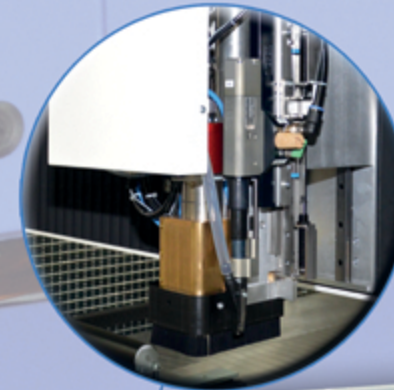
Routing unit to mill position holes/pockets in both flatbed and/or rotary dies
