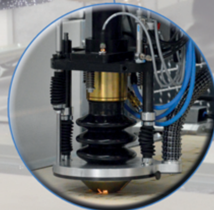
Standard cutting nozzle with crash protection system
