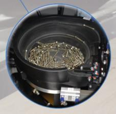
Screw hopper to feed screwing unit
