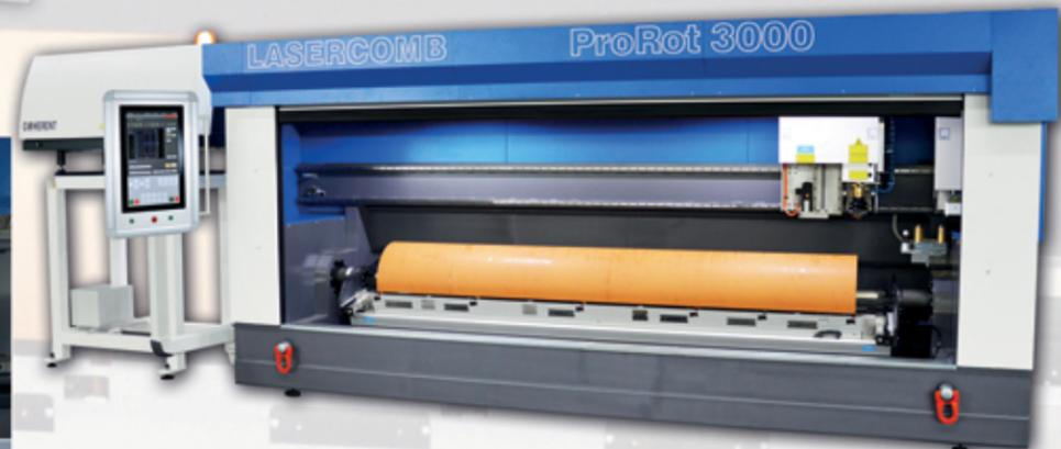
**Lasercutting systems for flatbed and rotary dieboard**
