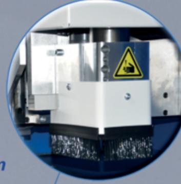
Standard cutting nozzle with crash protection system
