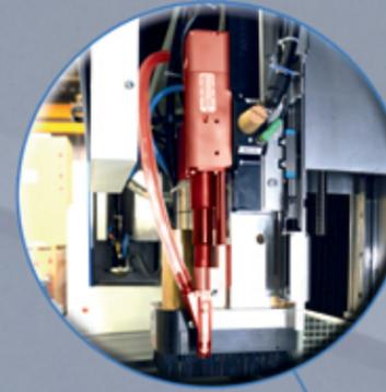
Routing unit to mill position holes/pockets
