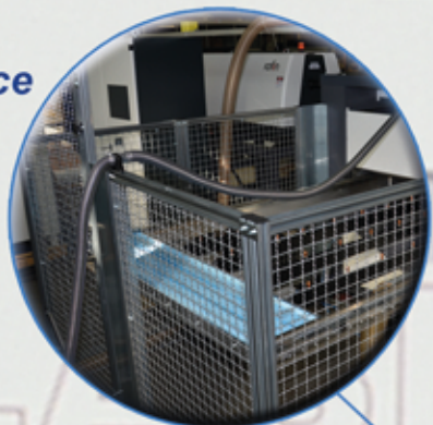
Water cooler for cooling of the lasersource and cutting optics
