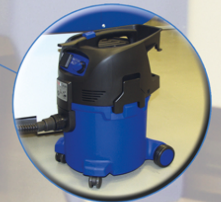
Waste extraction during pertinax milling via industrial type vacuum cleaner
