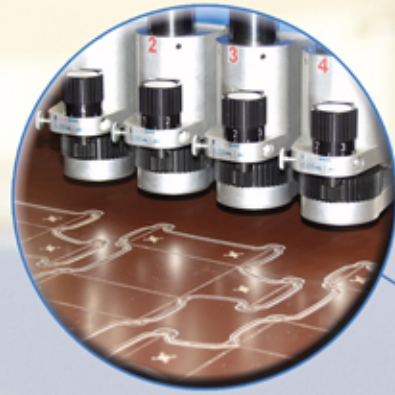
4 Spindle milling head with integrated dust extraction
