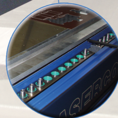
12/24 Tool rack for various routing bits used for pertinax/steel milling- automatic tool change
